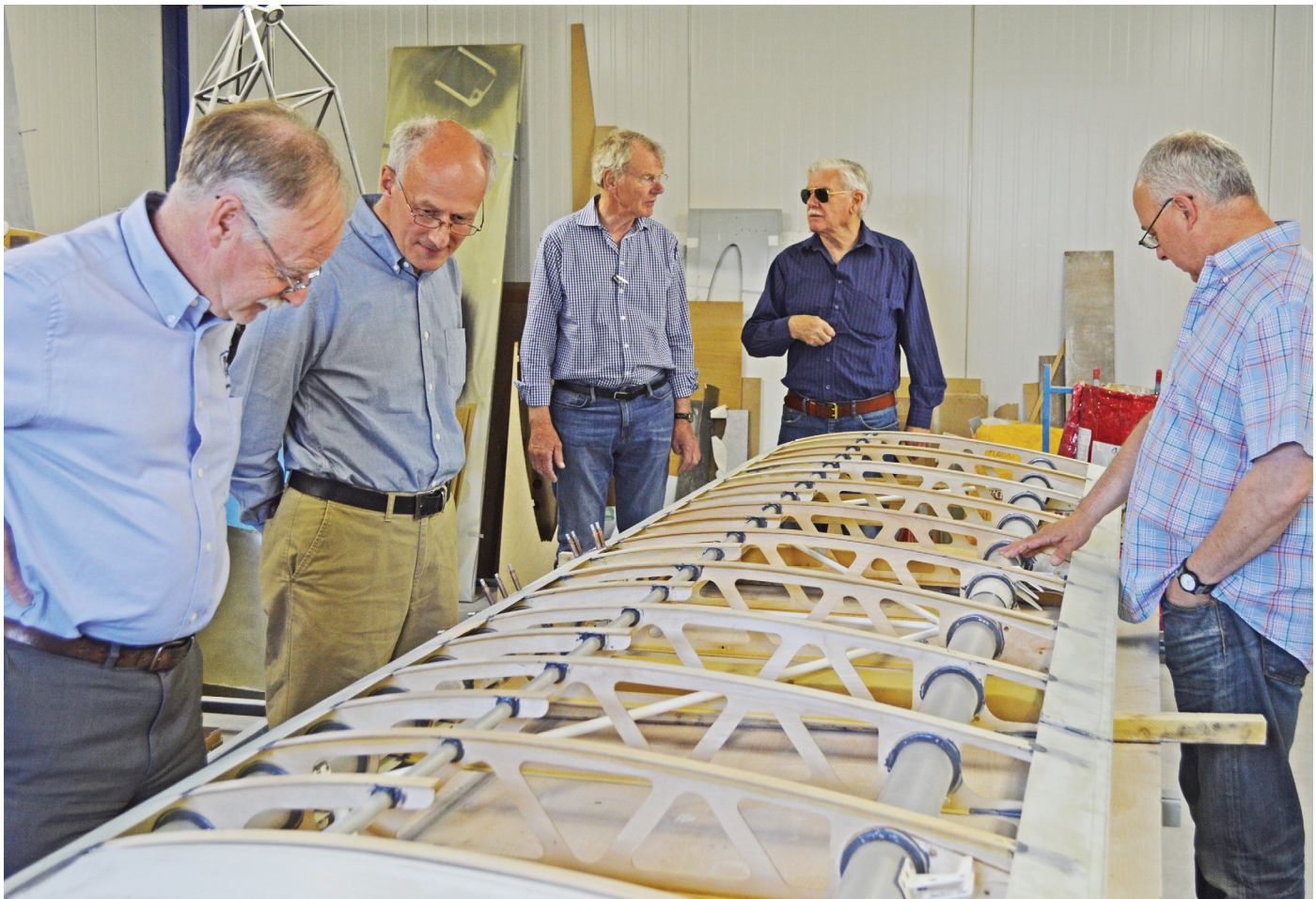
An M108 wing awaits the return of its builder to finally fettle and cover it in fabric.
