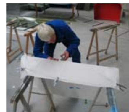
Clipping the fabric to the control surface before gluing
