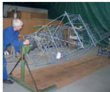
Fuselage mounted on rotatable jig for ease of access
