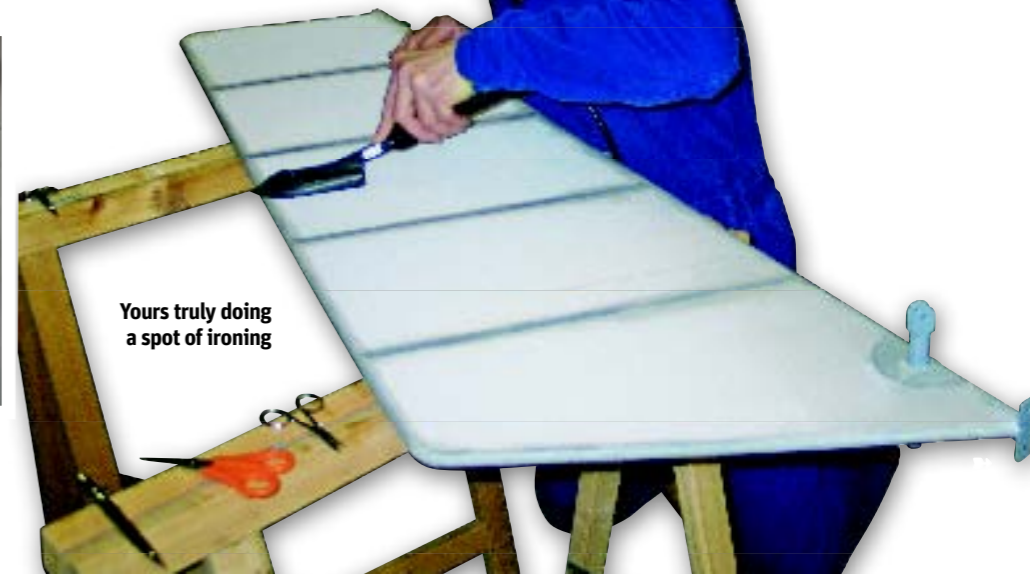
Clipping the fabric to the control surface before gluing
